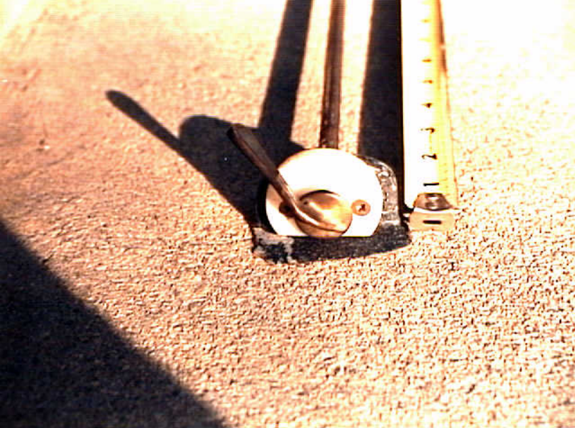
Photo 16. Fuel selector handle mounted in nylon block.
