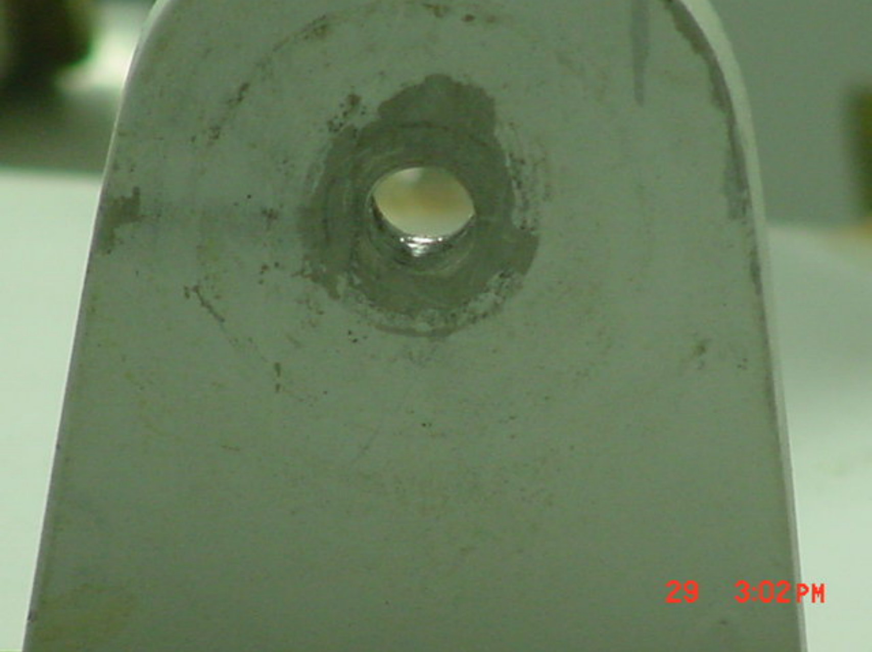
Photo 16. Canard Attachment Tab. Right Side
