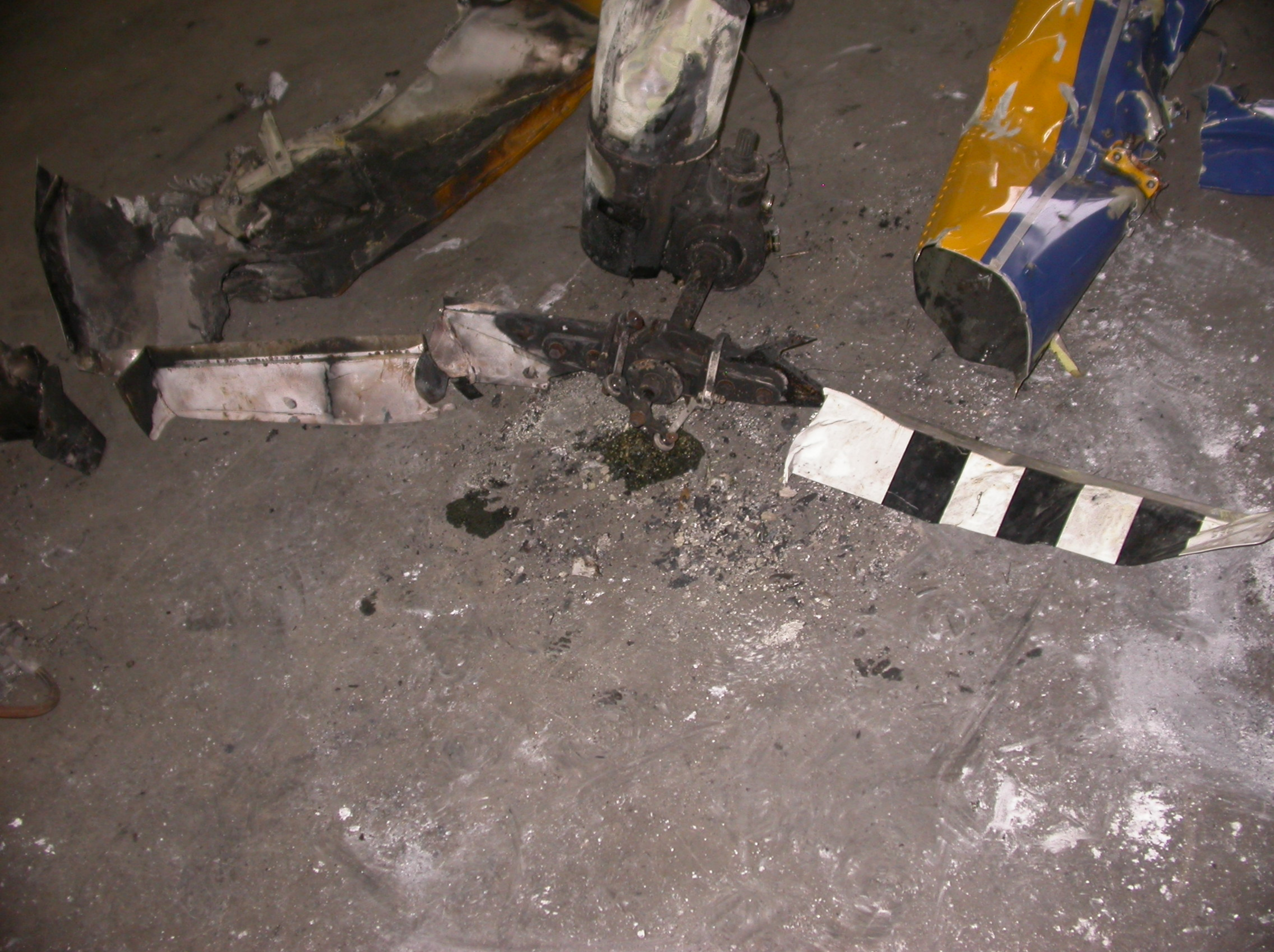
Photo 16) View of the Thermal and Impact damaged Tail Rotor Assembly. Photo by NTSB.
