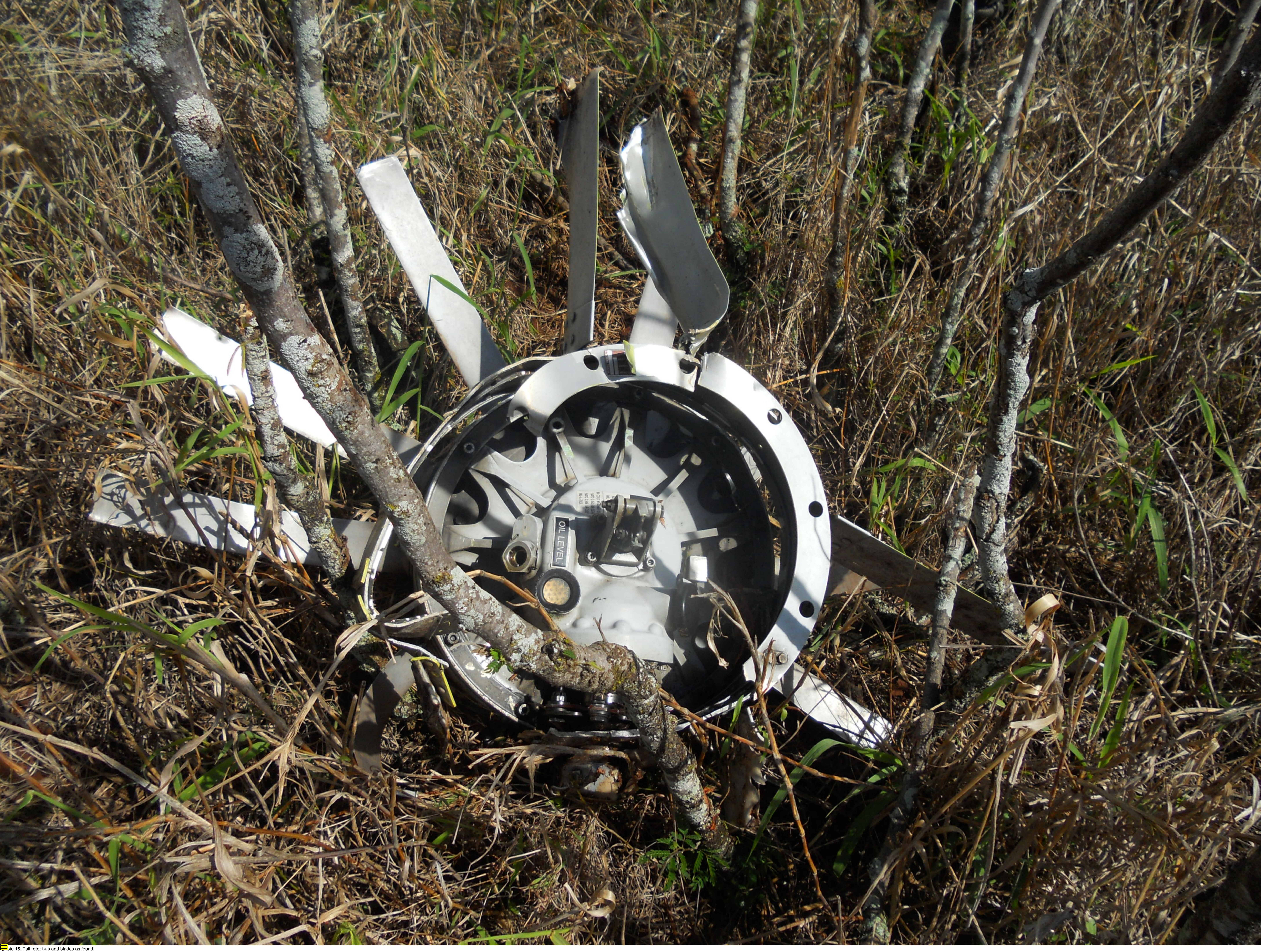
Photo 15. Tail rotor hub and blades as found.
