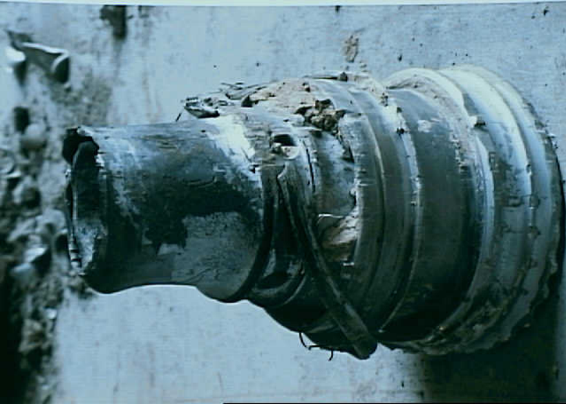
Photo 15. No. 2 engine fan shaft
