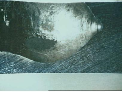
Photo 15. Hole adjacent to hole #1A drilled with HSS to failure by increased cutting data and without coolant. BEA has been performed.
