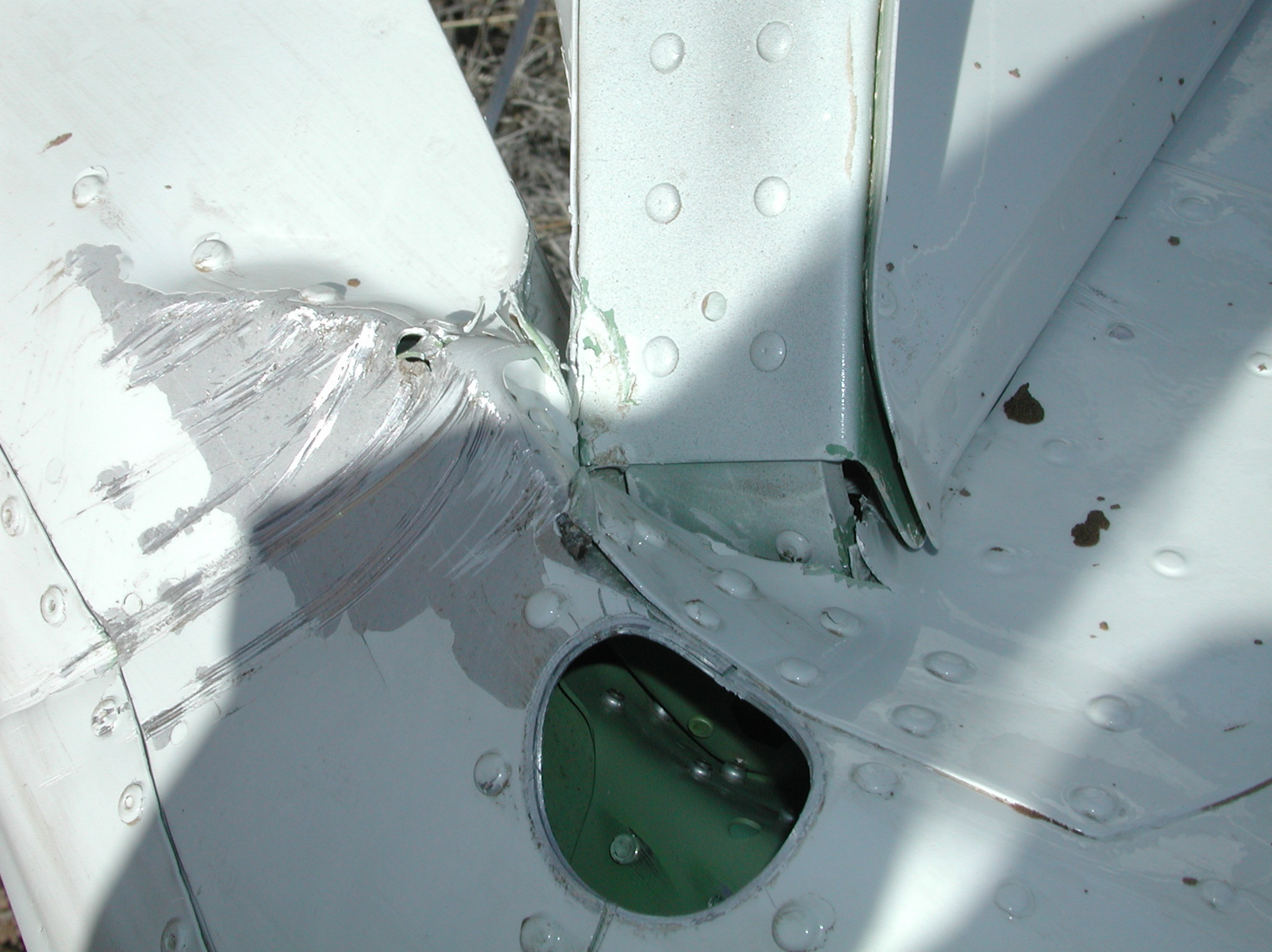
Photo 15: Top of vertical stabilizer with scratches and transfer material.
