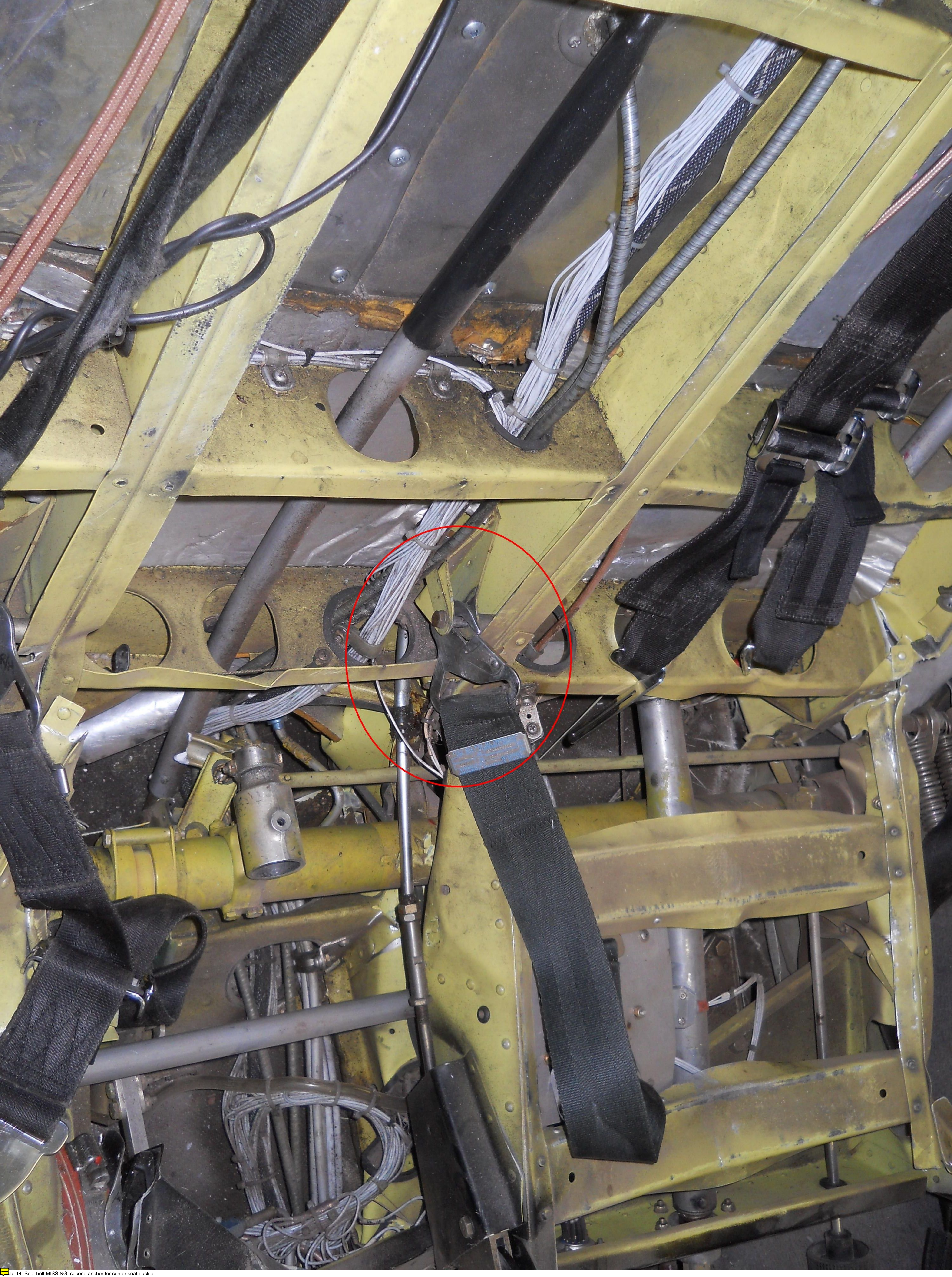
Photo 14. Seat belt MISSING, second anchor for center seat buckle
