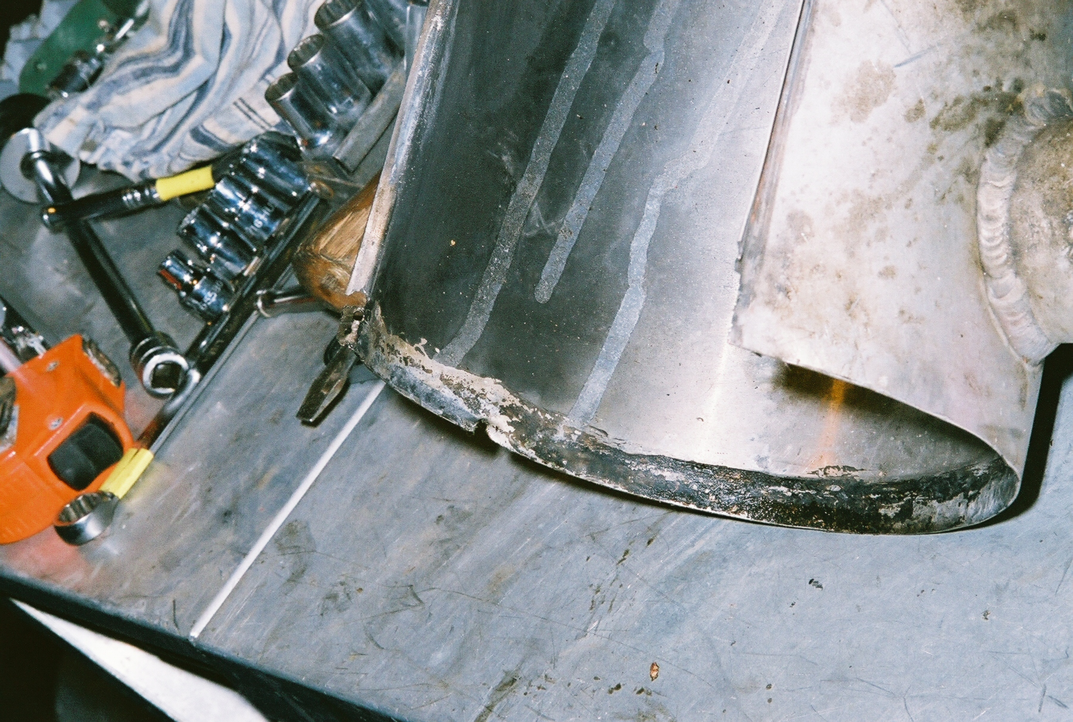
Photo 14. Heater muff showing location where material had been attached.
