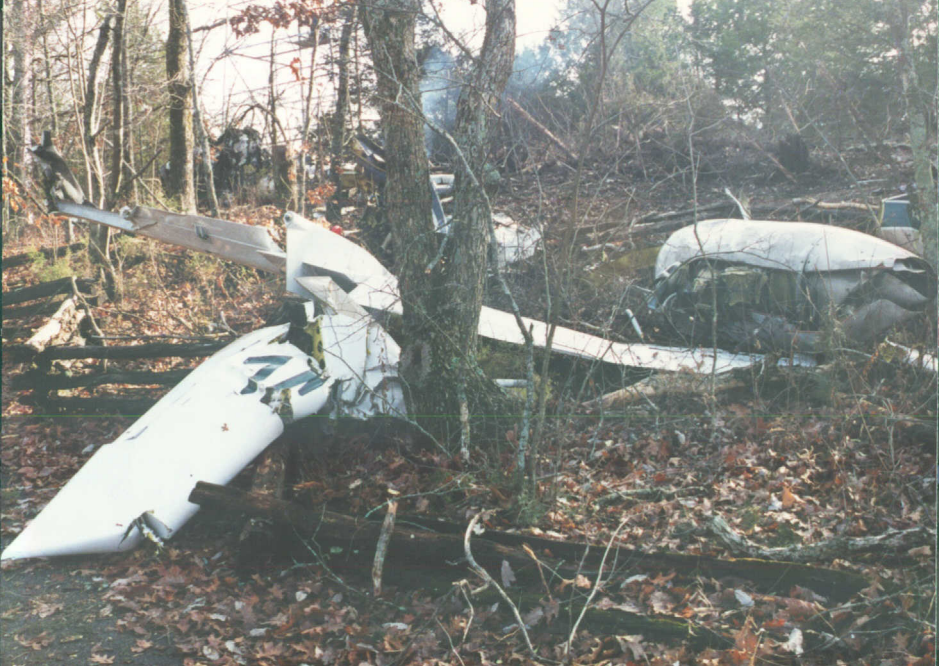
Photo 14. Empennage and Right Engine, Aft View
