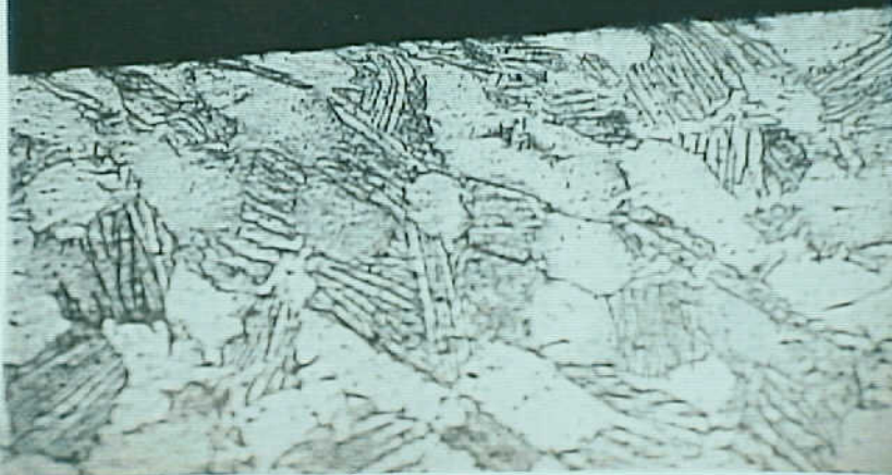
Photo 14. Cross section of hole #25 showing deformed material to a depth of 5 \mu\text{m} (0.20 mills). Mag 500X.
