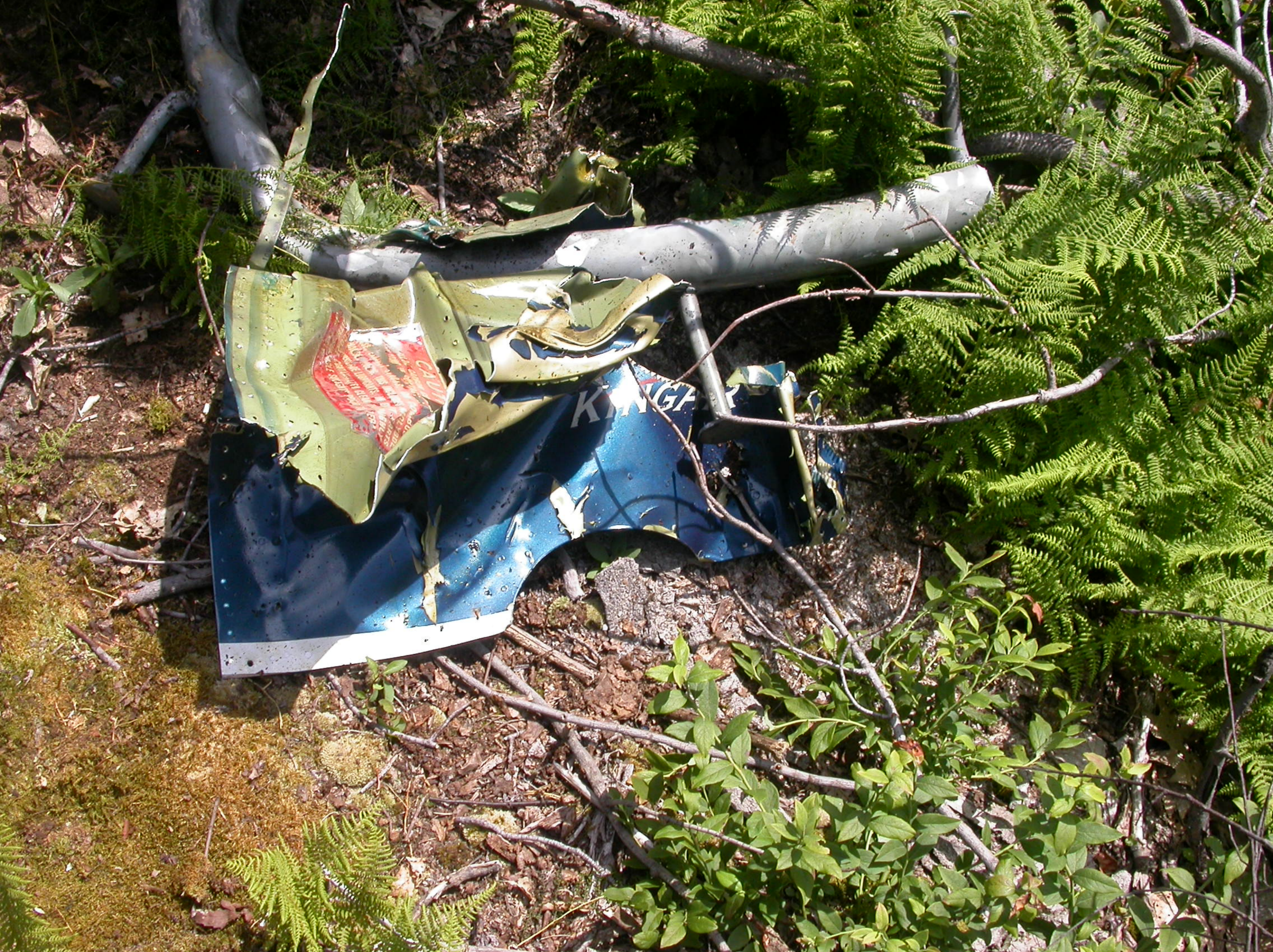
Photo 14: Antenna Beacon Mast with Portion of Right Engine Cowling
