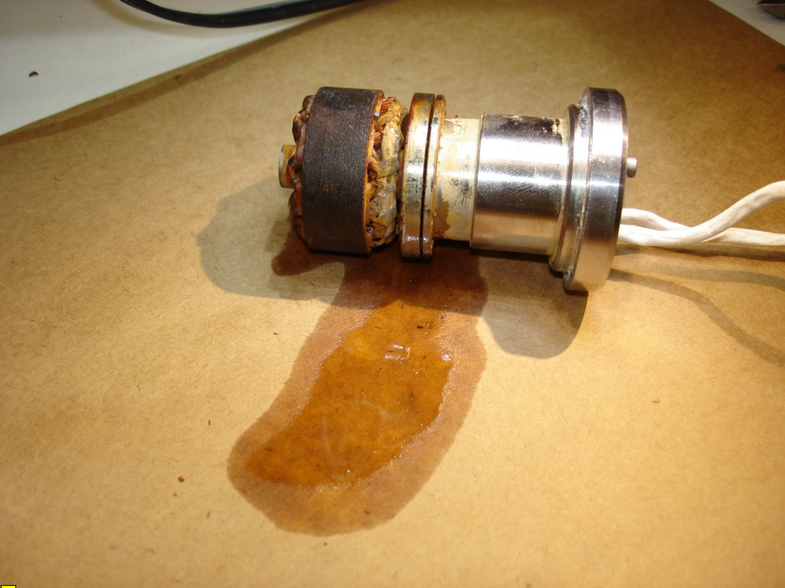
Photo 13. View of the stepper motor with the outer casing removed.
