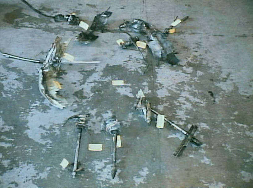
Photo 13. No. 1 engines reverser hydraulic actuators and TB/FW fragments
