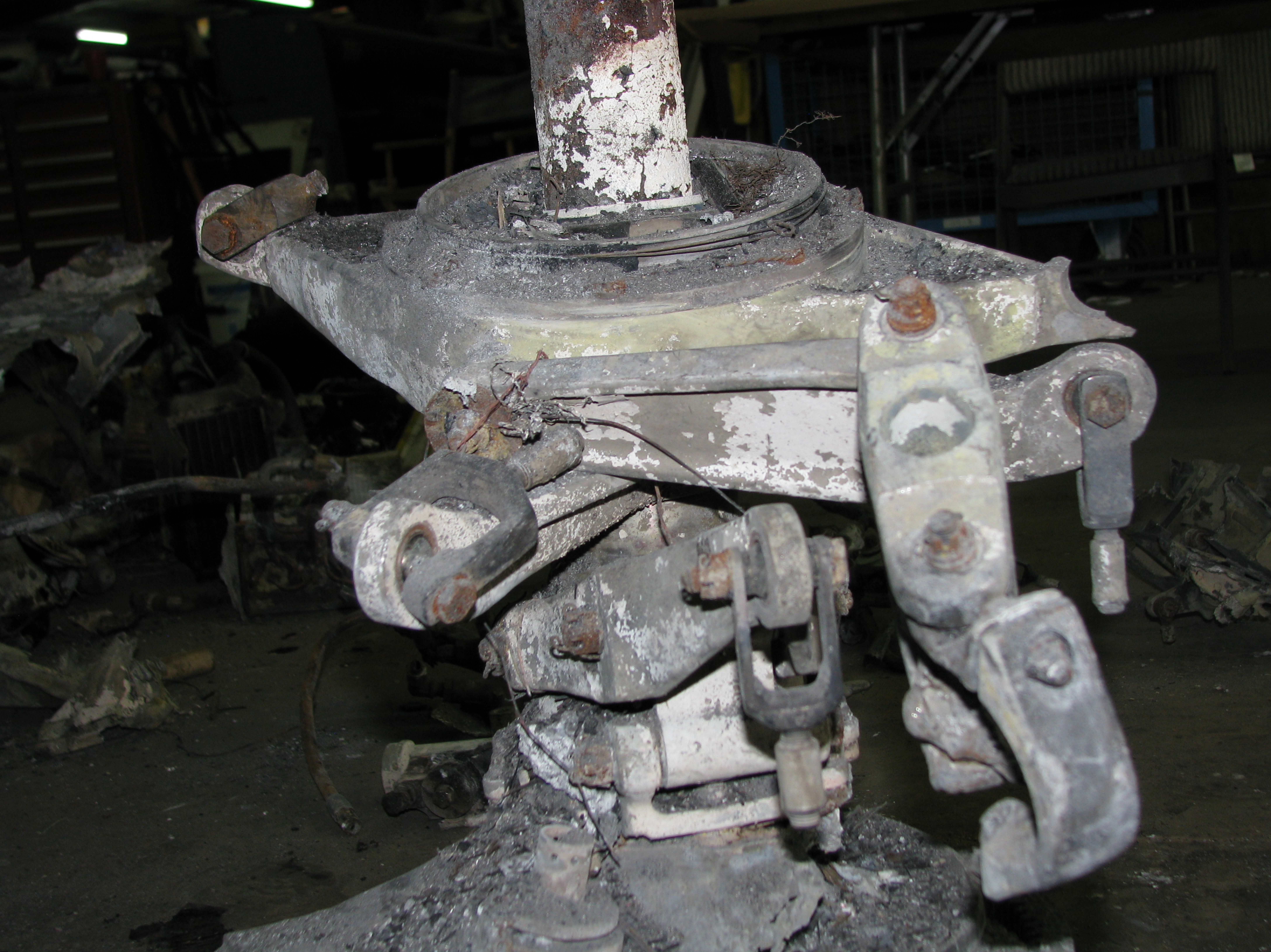
Photo 13) View of the Thermal Damaged Swashplate. Photo by Bell Helicopter.
