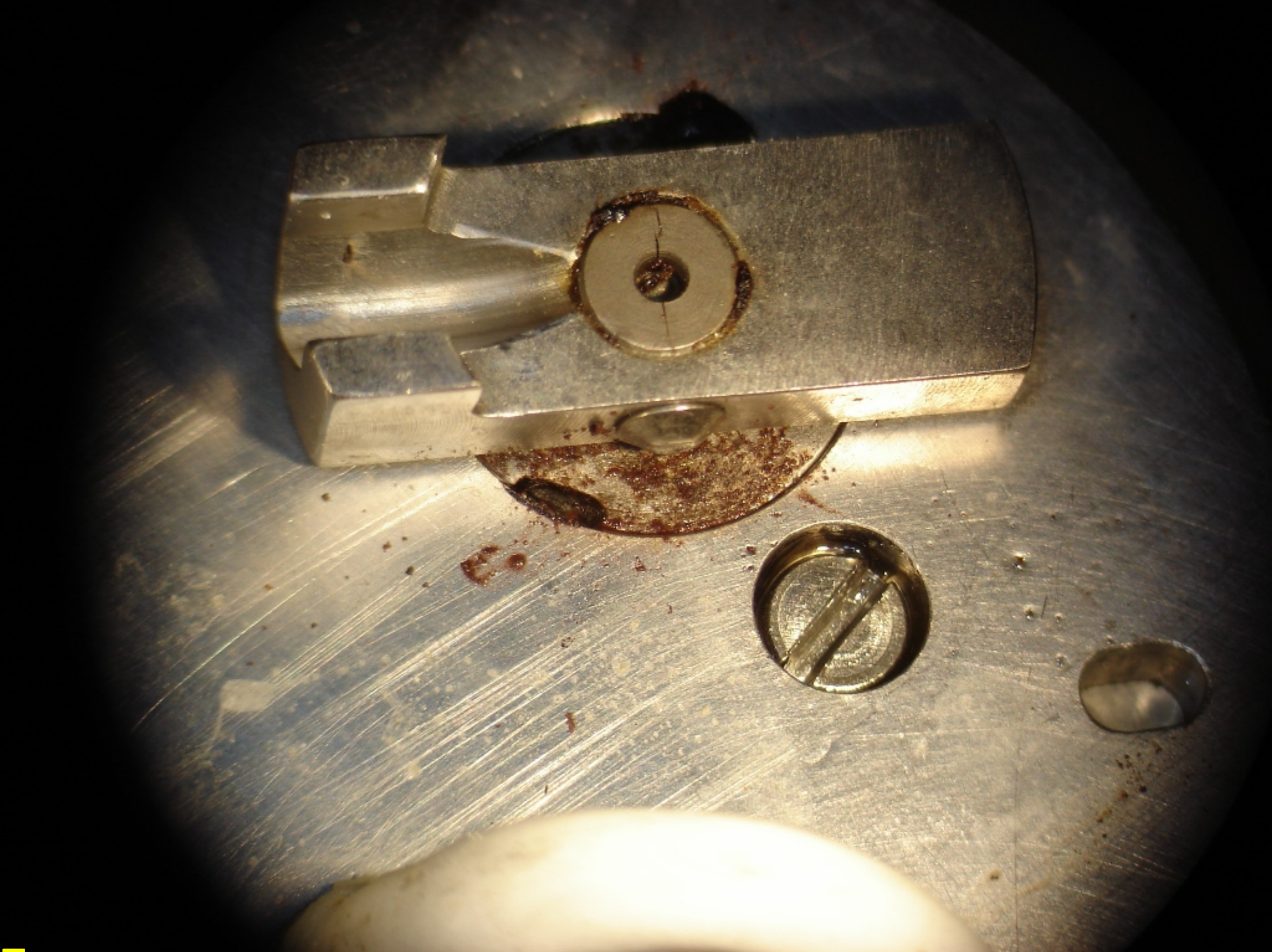
Photo 12. Stepper motor shaft with the crack visible.
