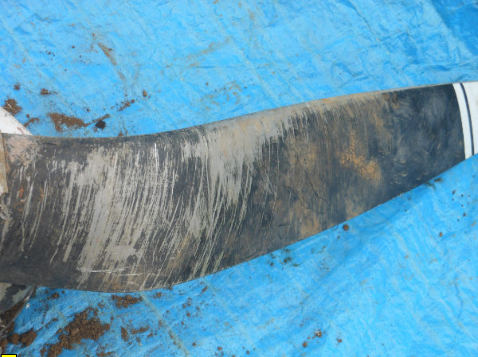
Photo 12. Propeller blade B, showing the chord-wise scarring on its cambered face.
