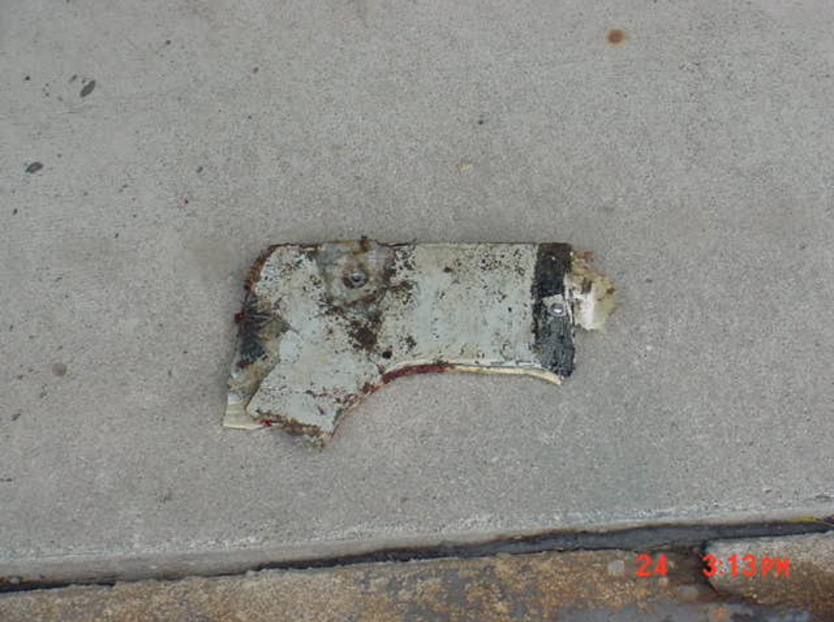
Photo 12. Piece of Forward Bulkhead (right side) With Canard imbedded bushing
