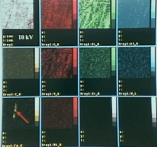
Photo 12. EDS map of the high intensity backscatter electron return from region 8, Figure 8. An elevated concentration of K-band iron (arrow) was observed.
