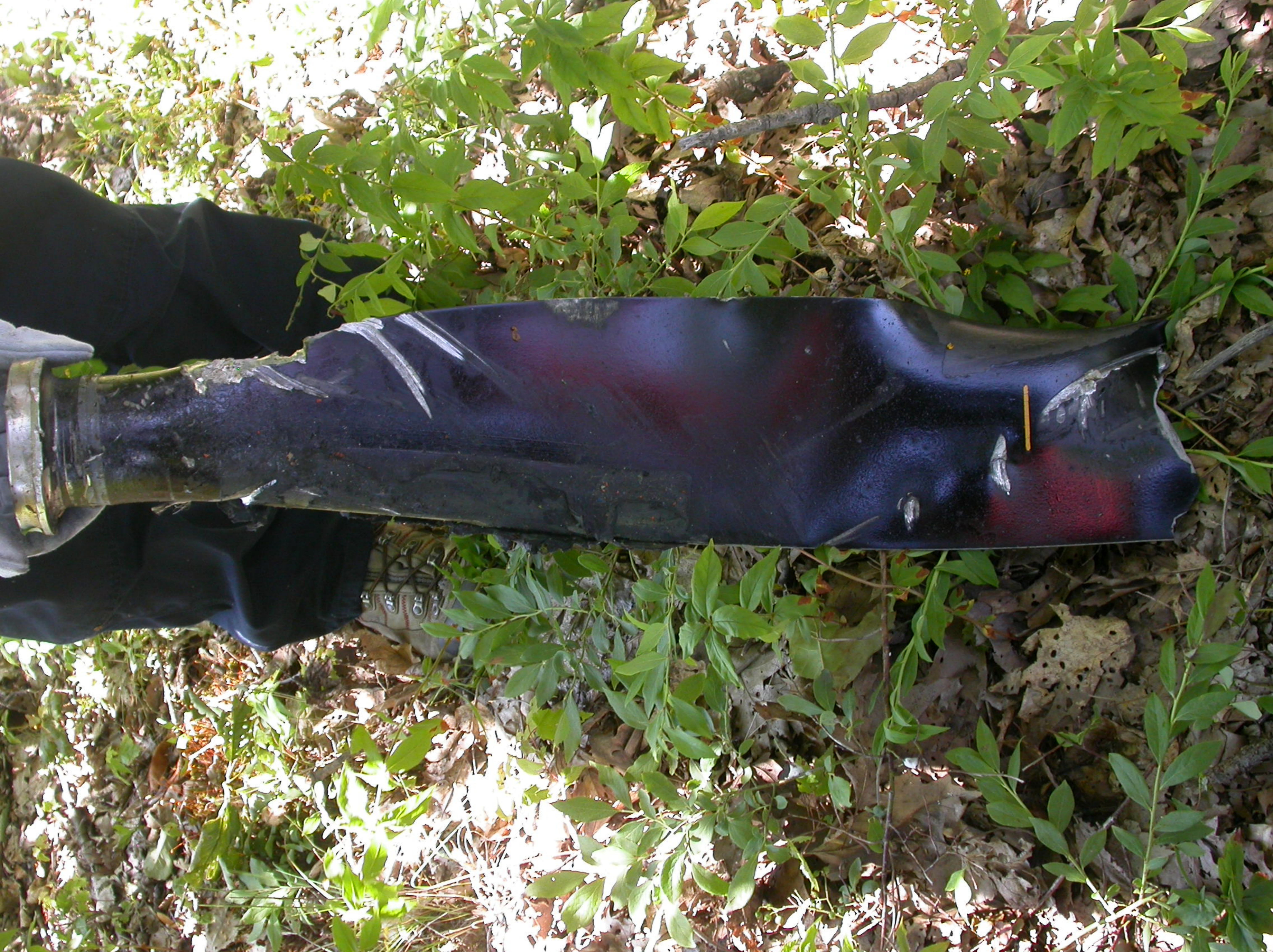
Photo 12: Propeller Blade From Right Propeller Showing Orange Transfer Marks
