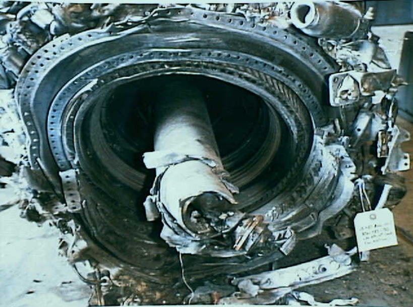
Photo 11. No. 1 engine LPT shaft and aft HPC case.
