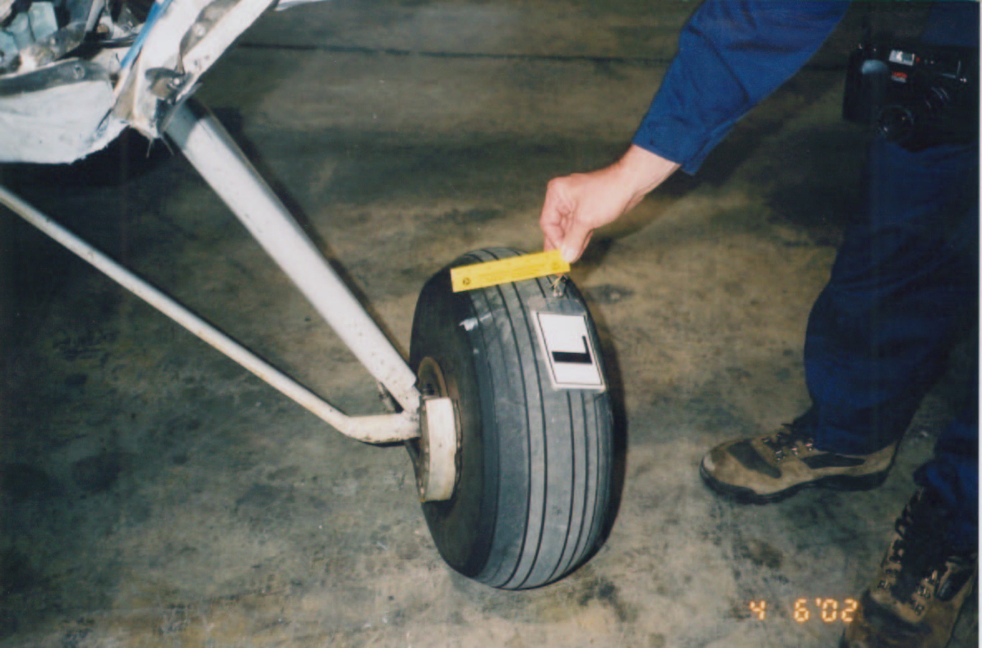
Photo 11 - Faint paint transfer of maroon paint on N5293H left main landing gear
