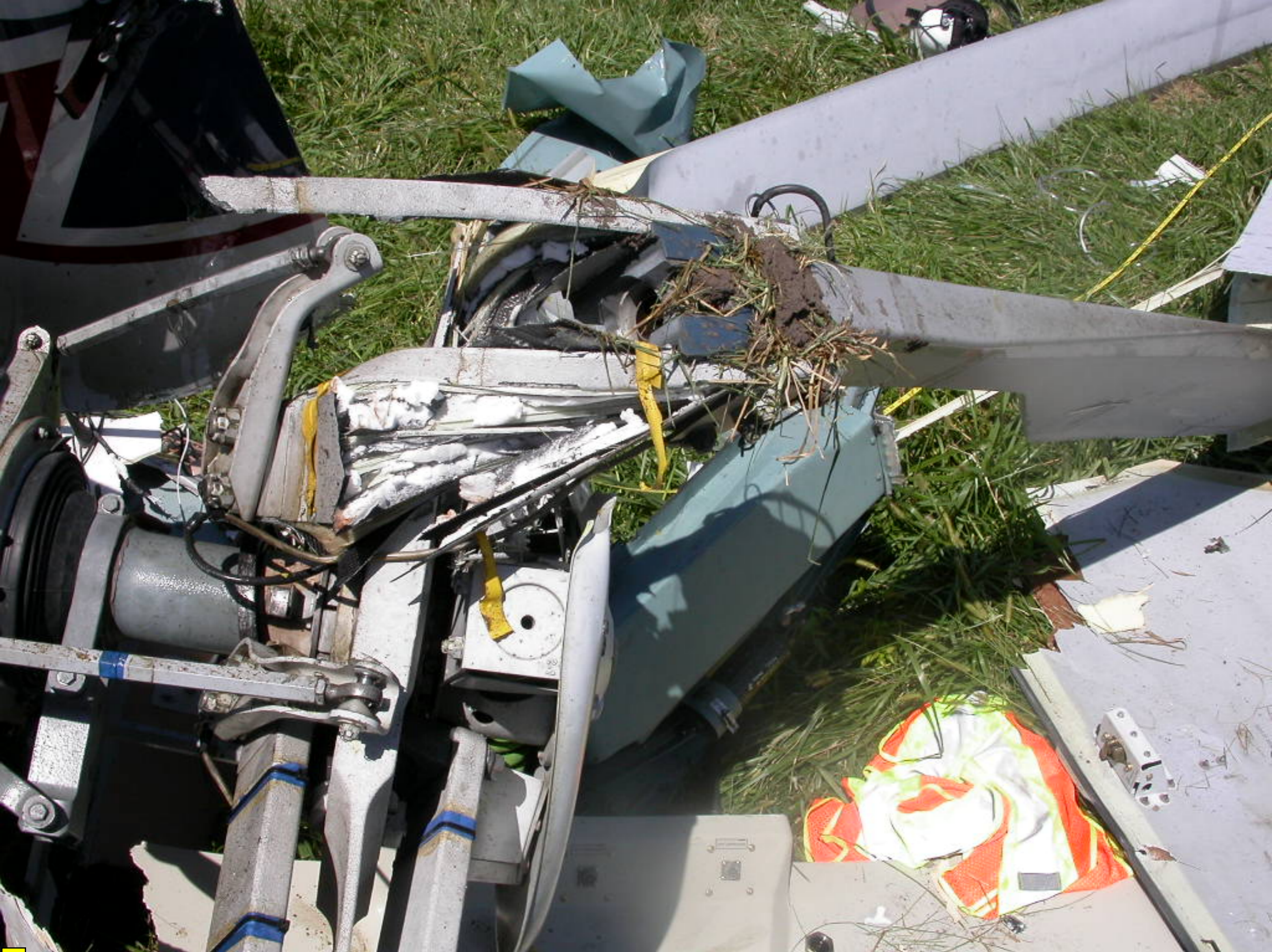
Photo 11: View of the main rotor hub with broken blades at the hub
