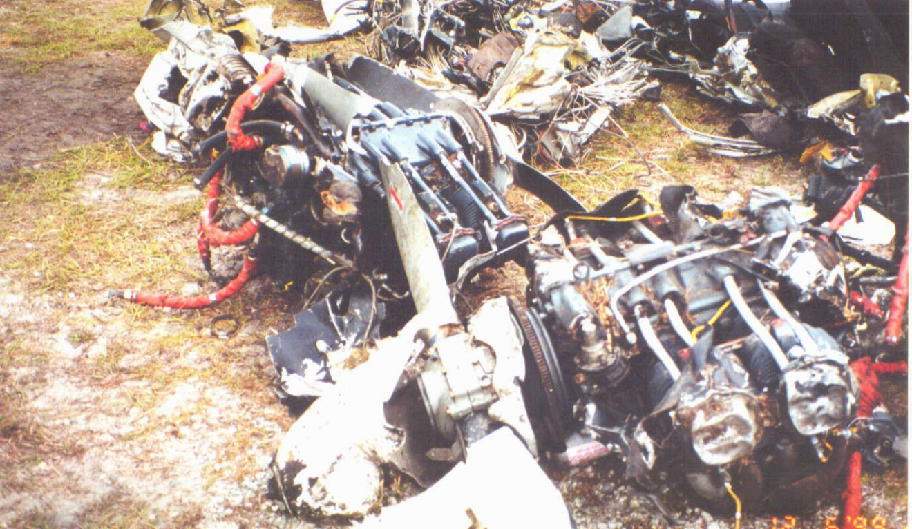
Photo 11: View of the left engine and fractured propeller blade of the Seminole matching impact signatures on the top of the engine of the Cadet
