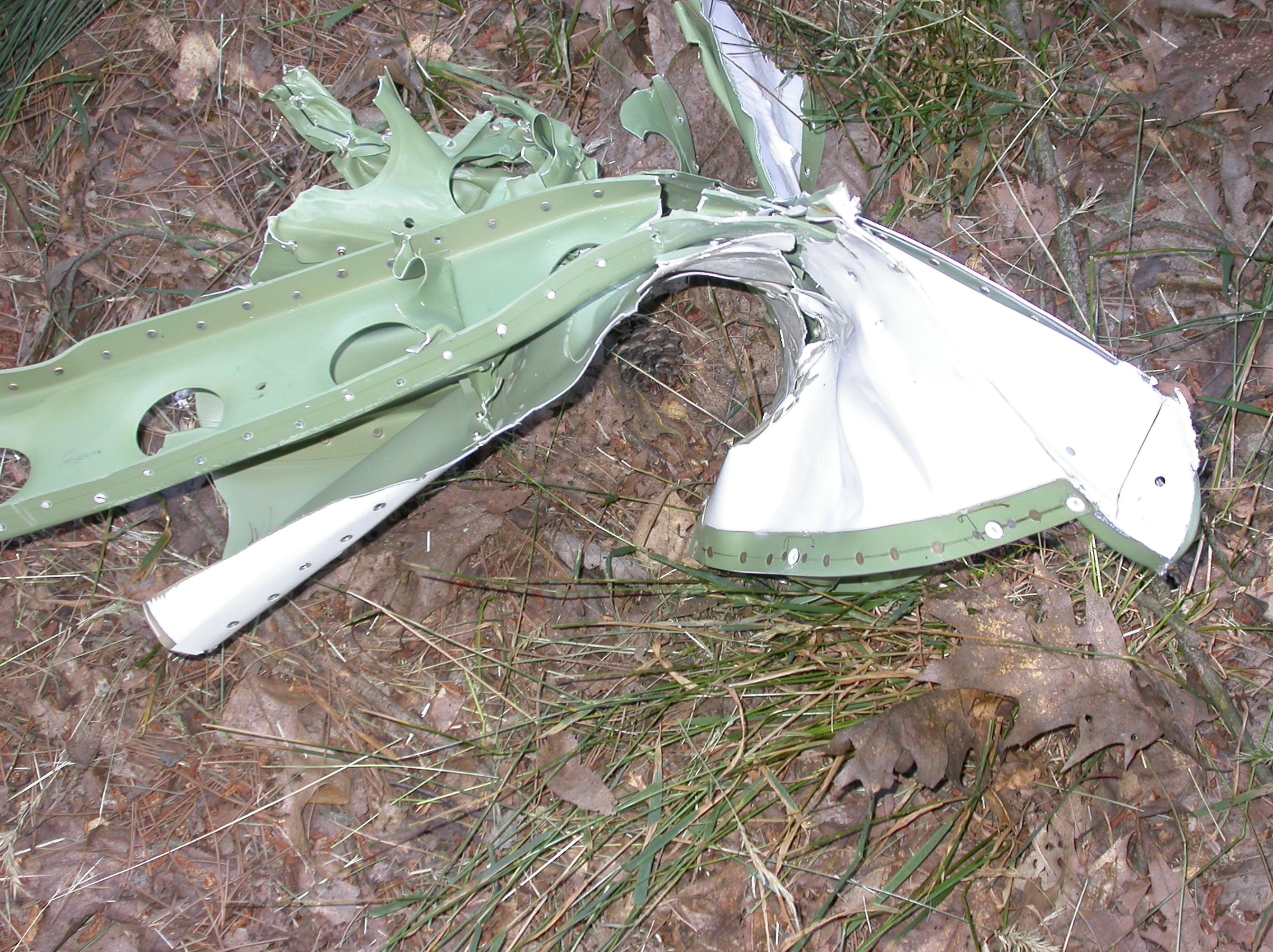
Photo 11: Portion of Right Wing Structure Showing Concave Depression.
