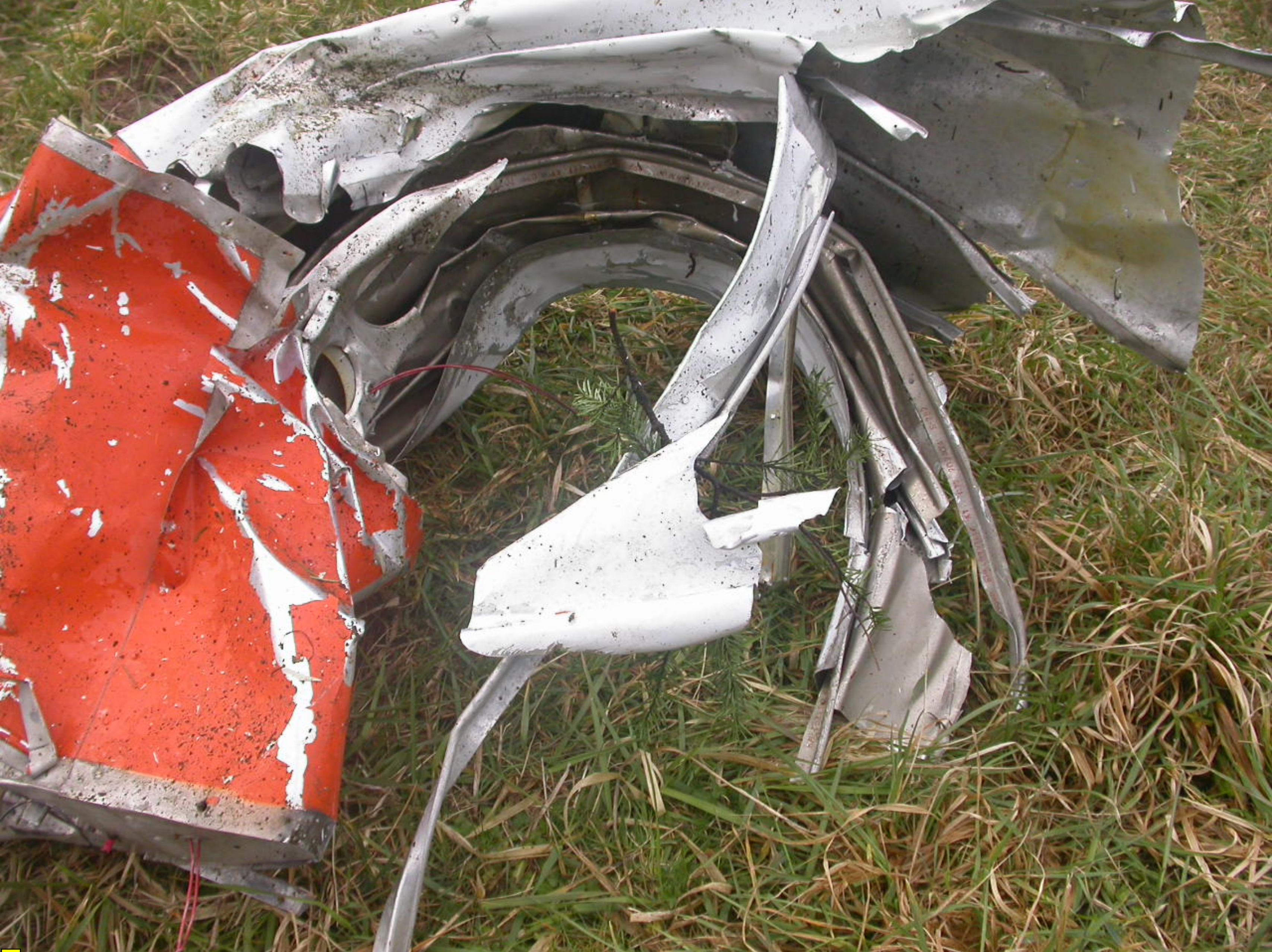
Photo 10. Semicircular indentation in the separated portion of the right wing.
