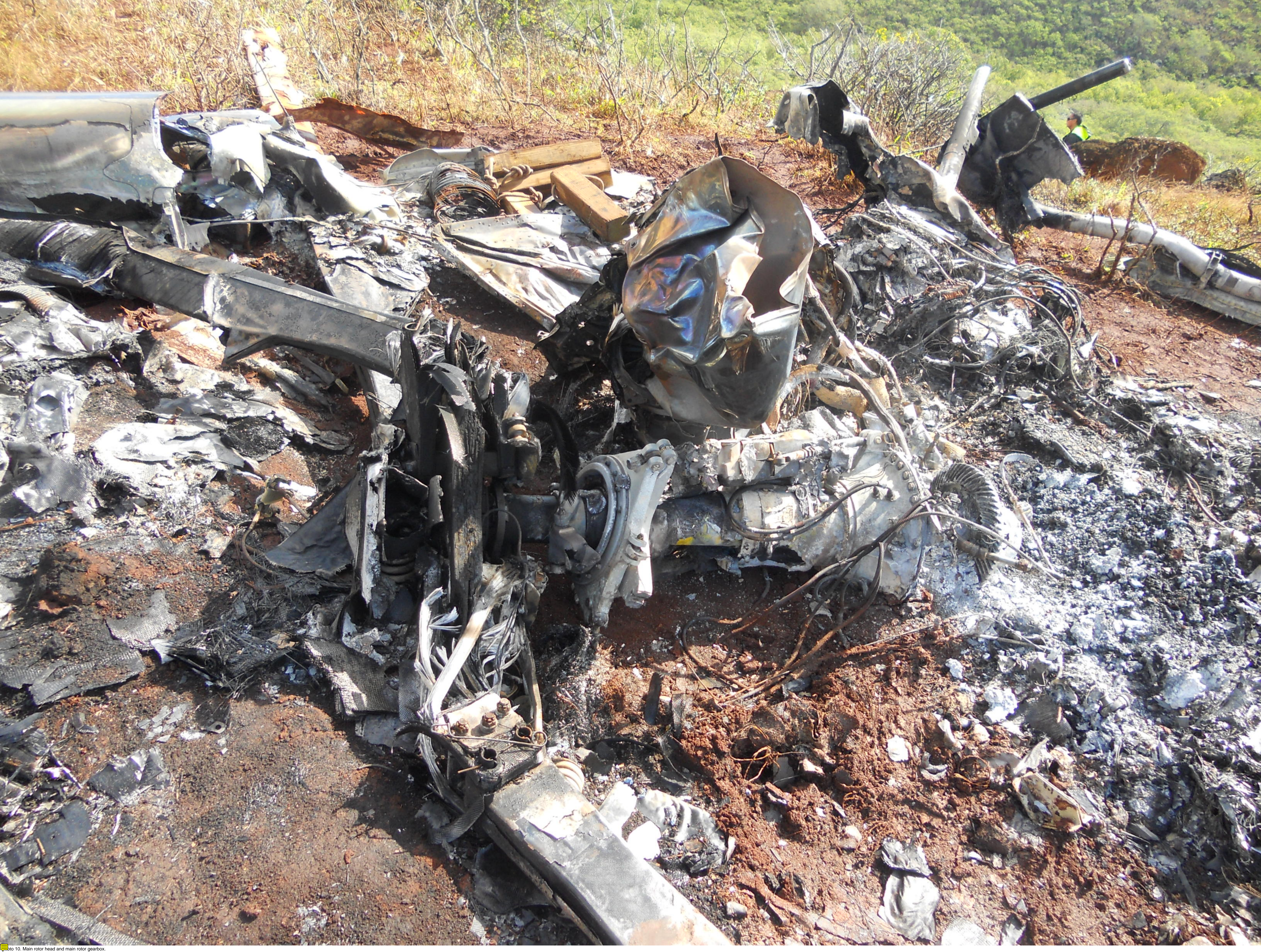
Photo 10. Main rotor head and main rotor gearbox.
