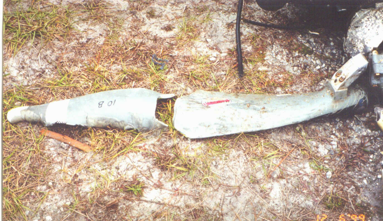
Photo 10: View of the fractured propeller blade from the left propeller of the Seminole
