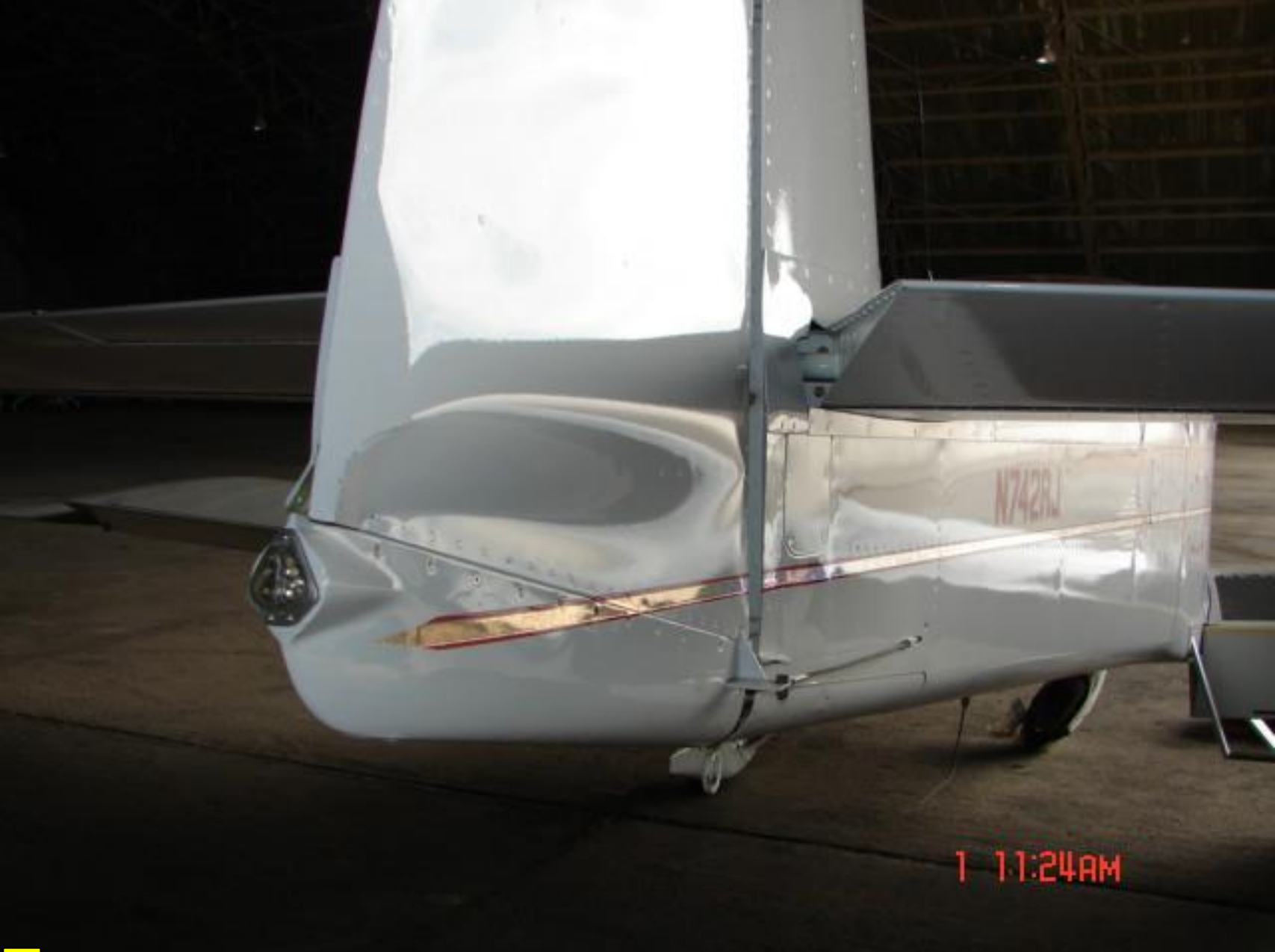
Photo 1. Damage to the rudder stiffener. Pilot
