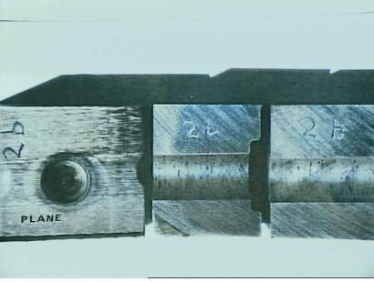
Photo 1. Hole #2B. Cutting without coolant with HSS drill to breakdown. Cutting data see report 9634-0101.
