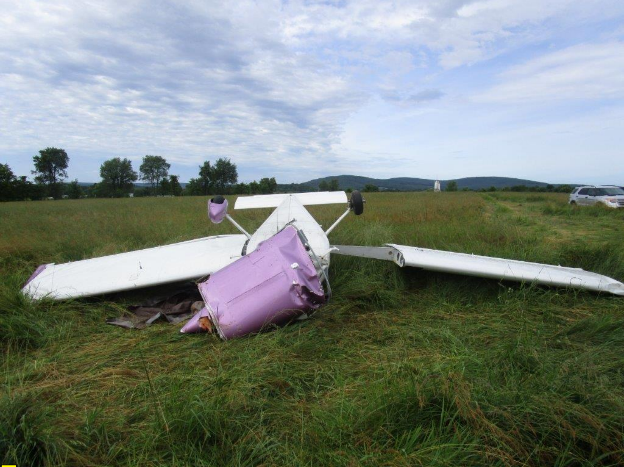
Photo 1-View of firewall damage (photo courtesy of the FAA)
