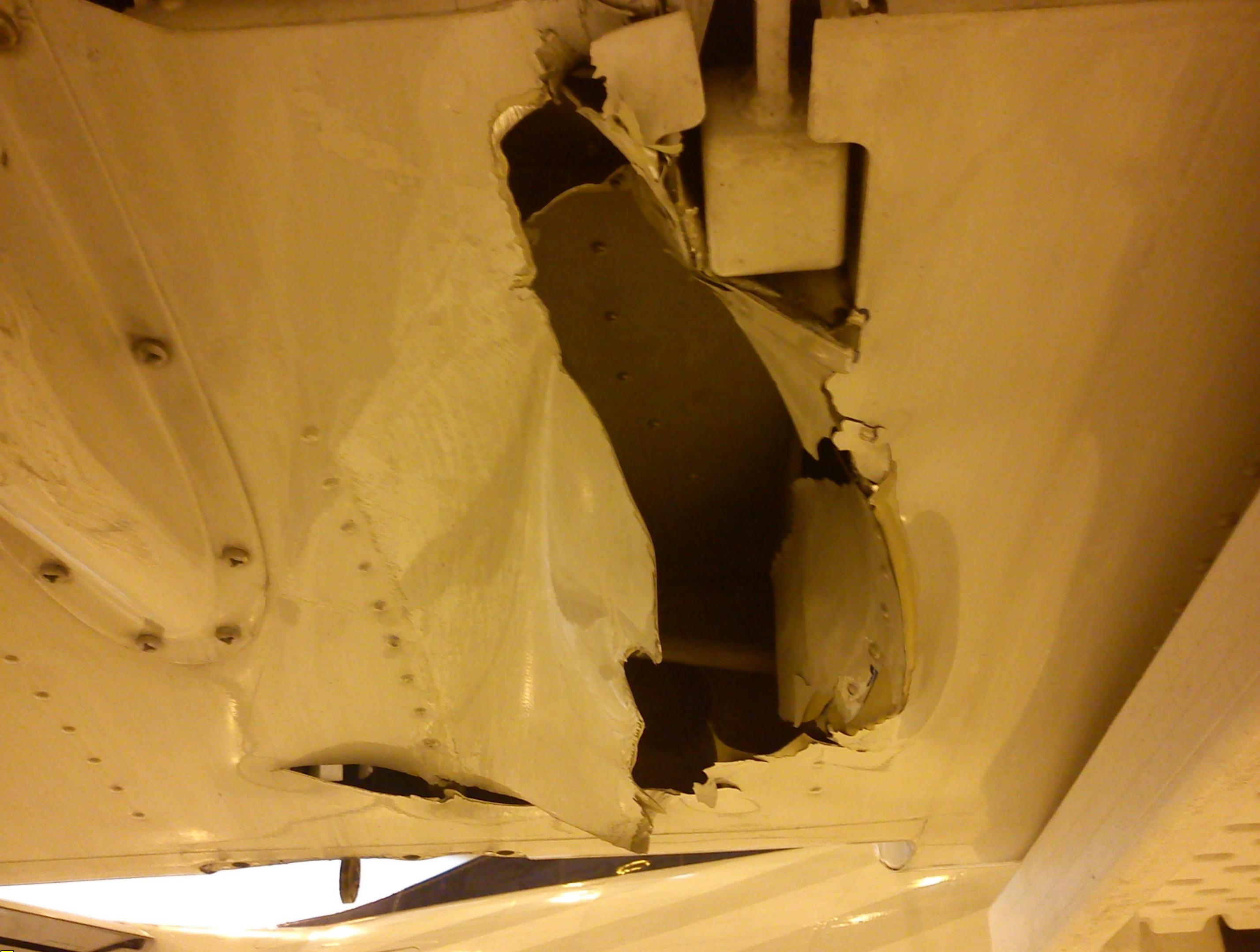
Photo 1- FAA photo-Elevator damage underside
