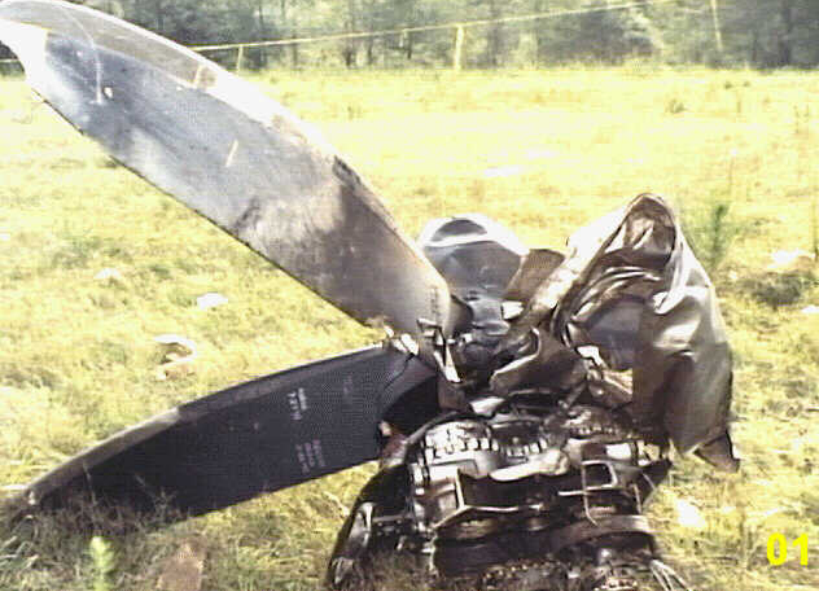
Photo 1 Left Engine and Propeller-Propeller and Reduction Gearbox at accident site.
