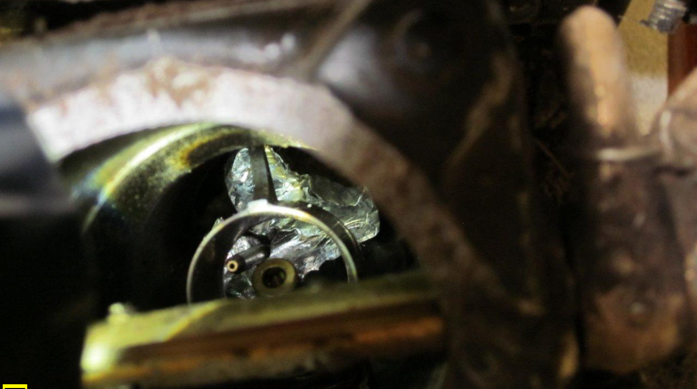
Photo 1 Debris Lodged Beneath Carburetor Venturi
