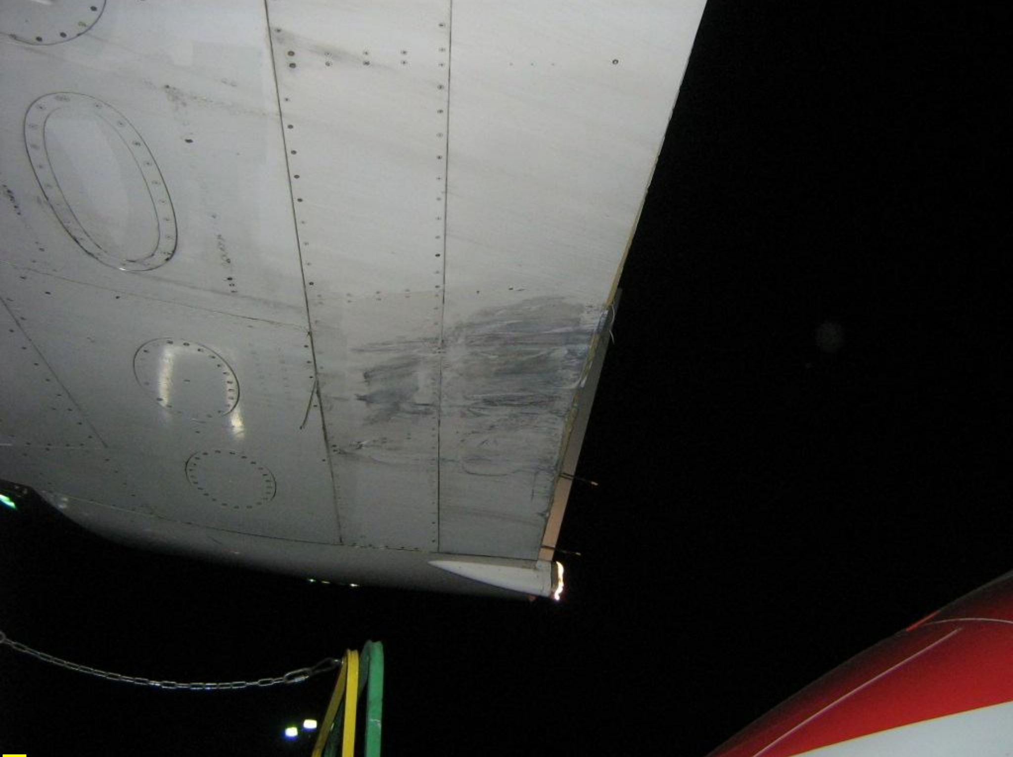
Photo 1 - Right wing damage to N945AN, Boeing 737-823
