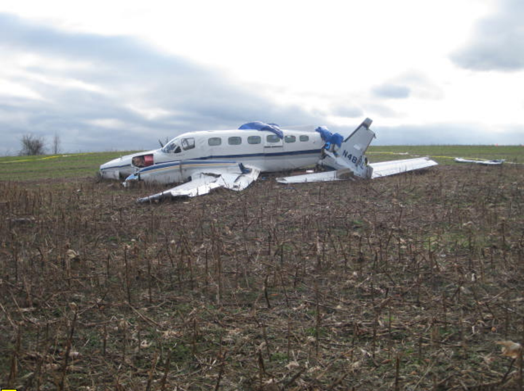
Photo 1 - Left Side of Airplane; Tail Broken to the Left and Left Wing Broken Forward
