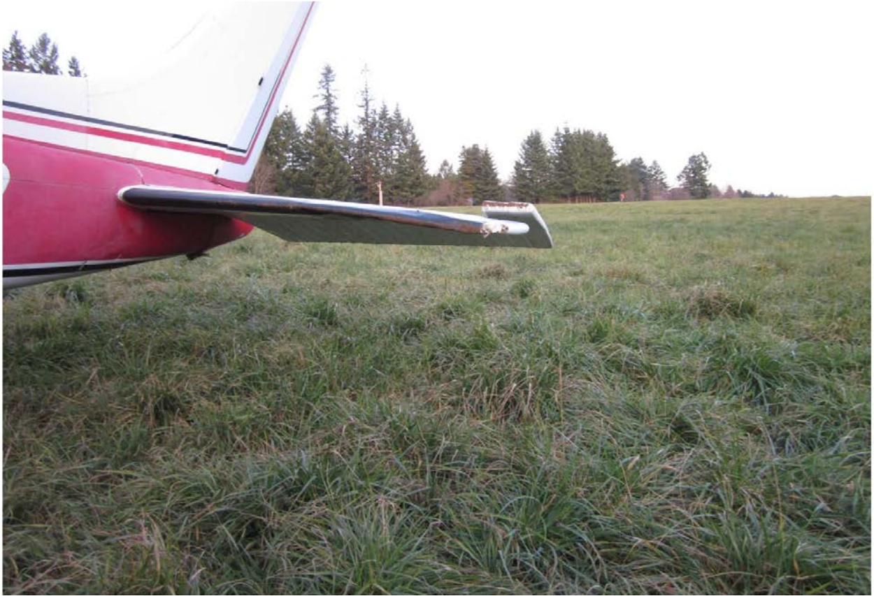
Photo 1: Damaged Left Side Horizontal Stabilizer (FAA)
