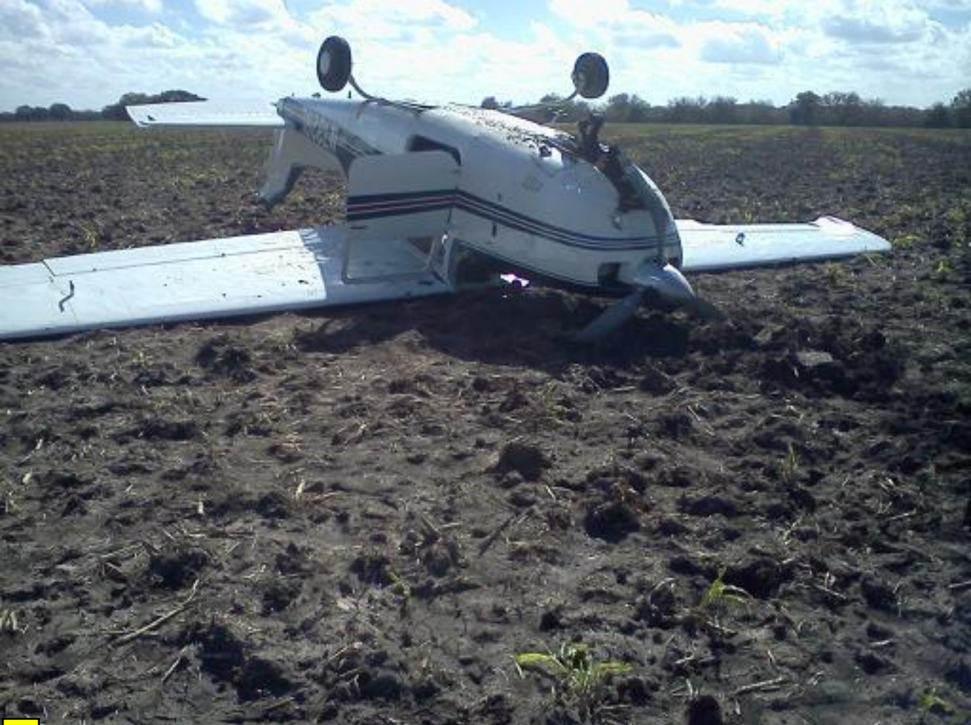
Photo – View of Inverted Wreckage at the Accident Scene (FAA Photo)
