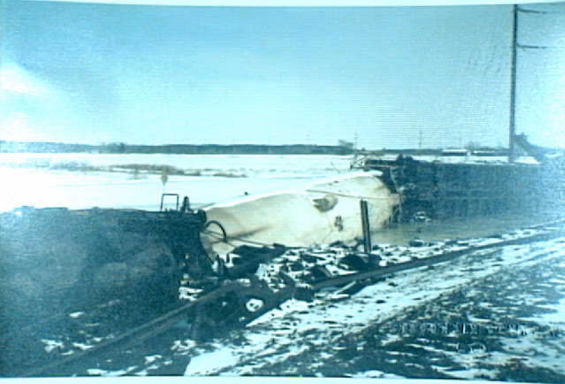
Photo 1: View of the derailed cars in the eastern section of the derailment site.
