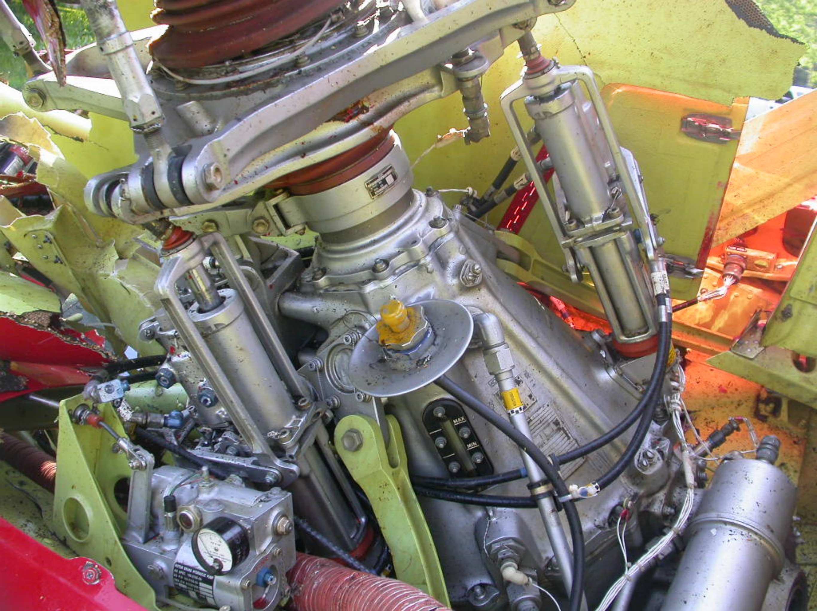
Photo 08. The transmission, cyclic- collective controls, and hydraulic accumulators.
