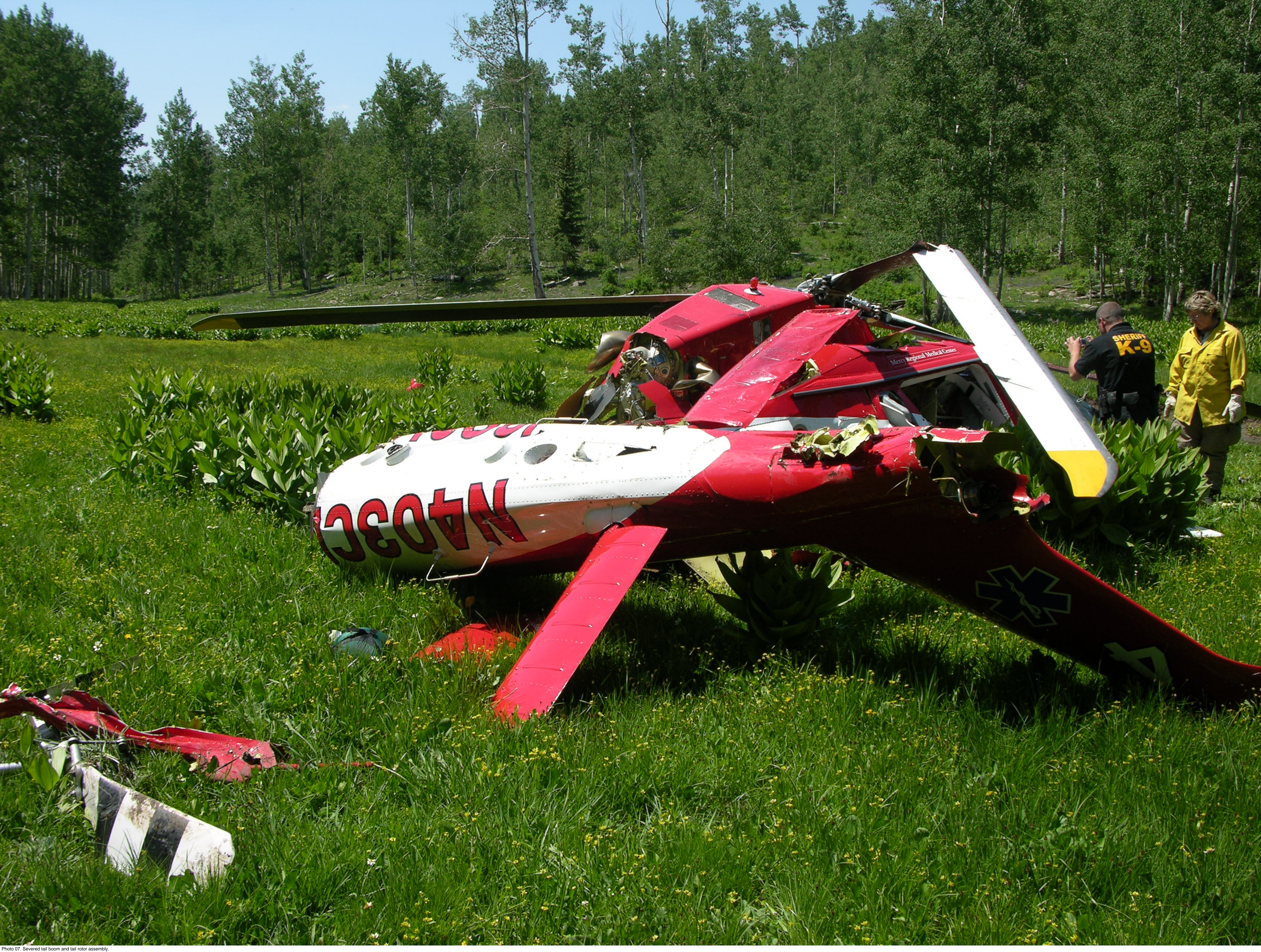
Photo 07. Severed tail boom and tail rotor assembly.
