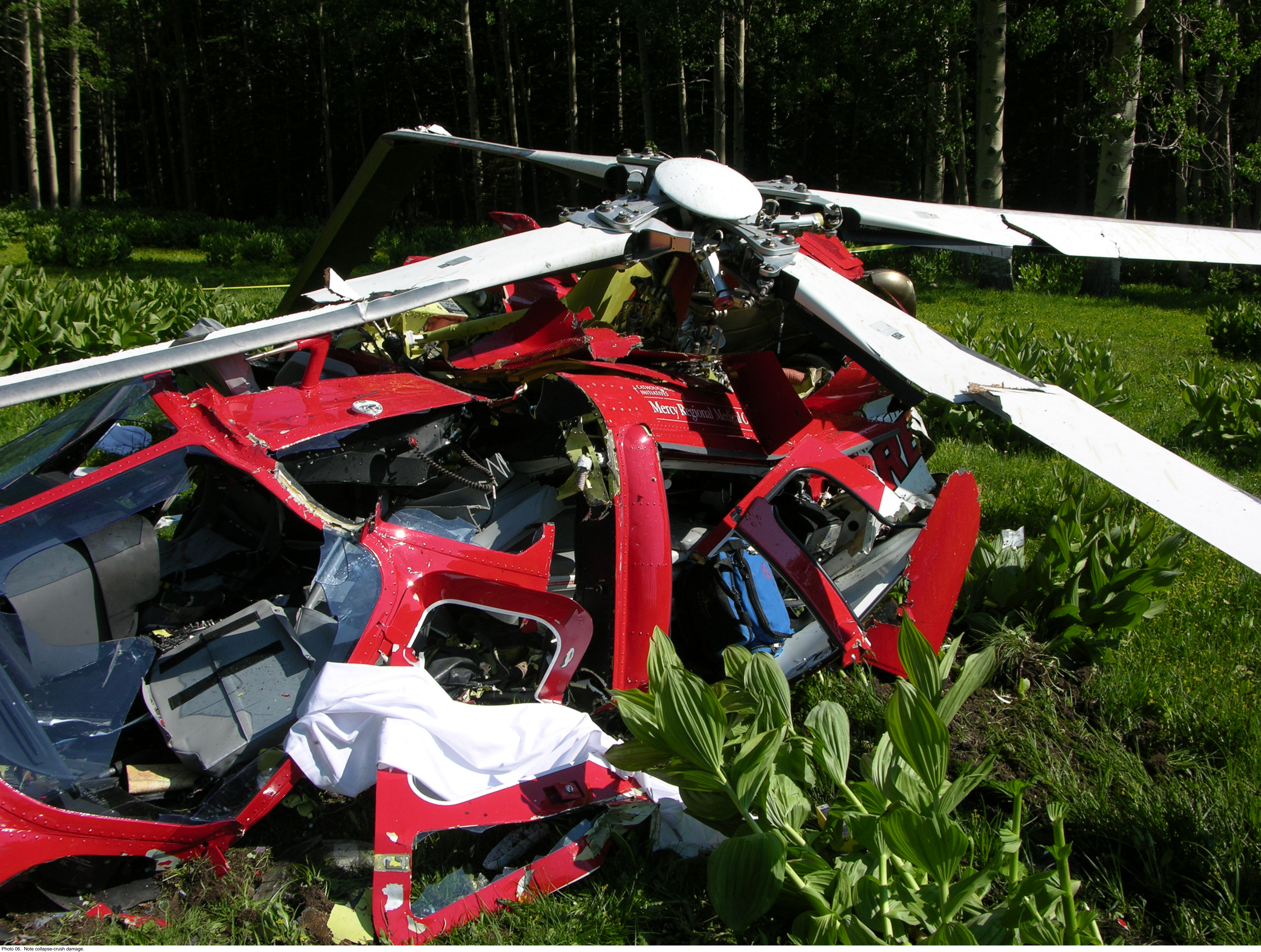
Photo 06. Note collapse-crush damage.
