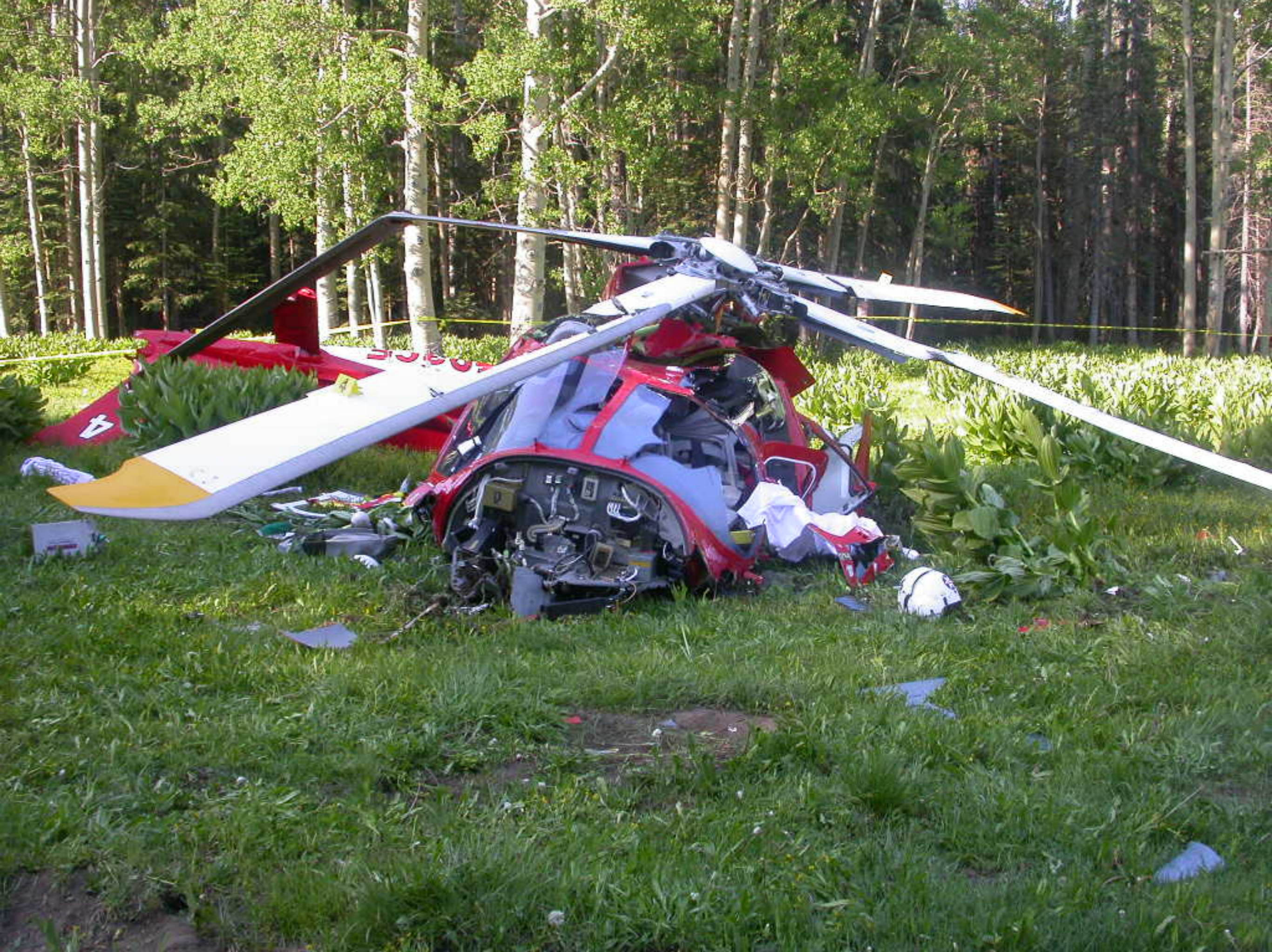
Photo 05. View to the south and nose of helicopter. Note crushed nose section and rotor blades.
