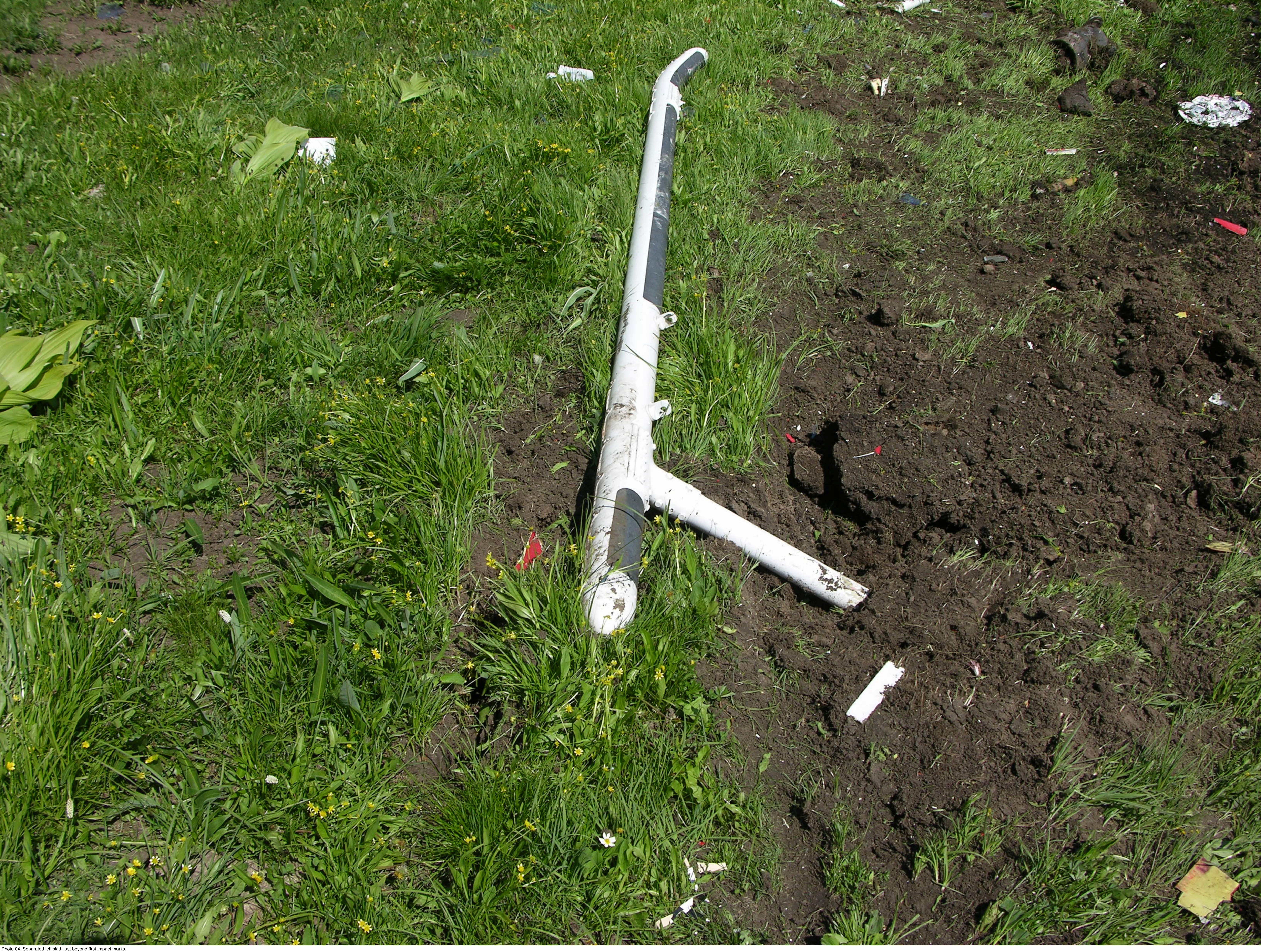
Photo 04. Separated left skid, just beyond first impact marks.
