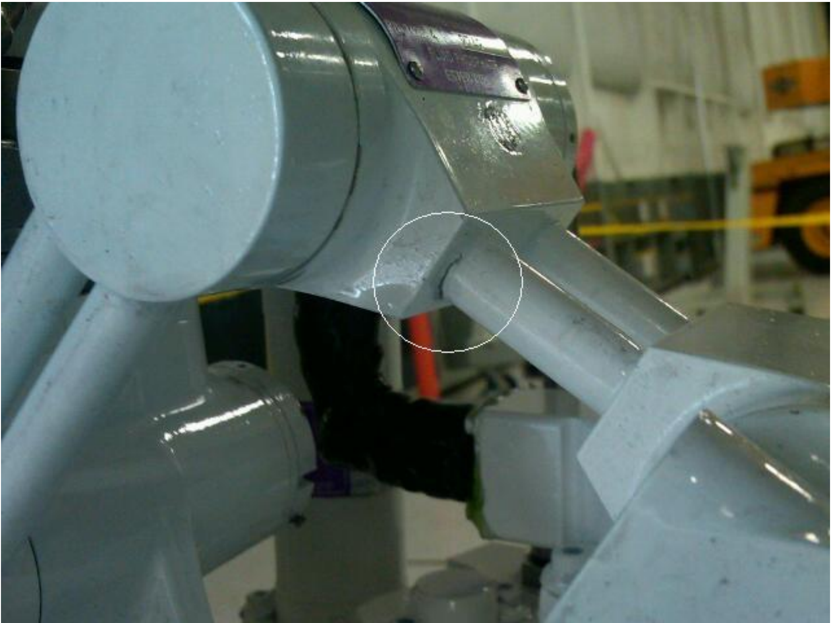
Photo View of the Cracked Swivel Tube
