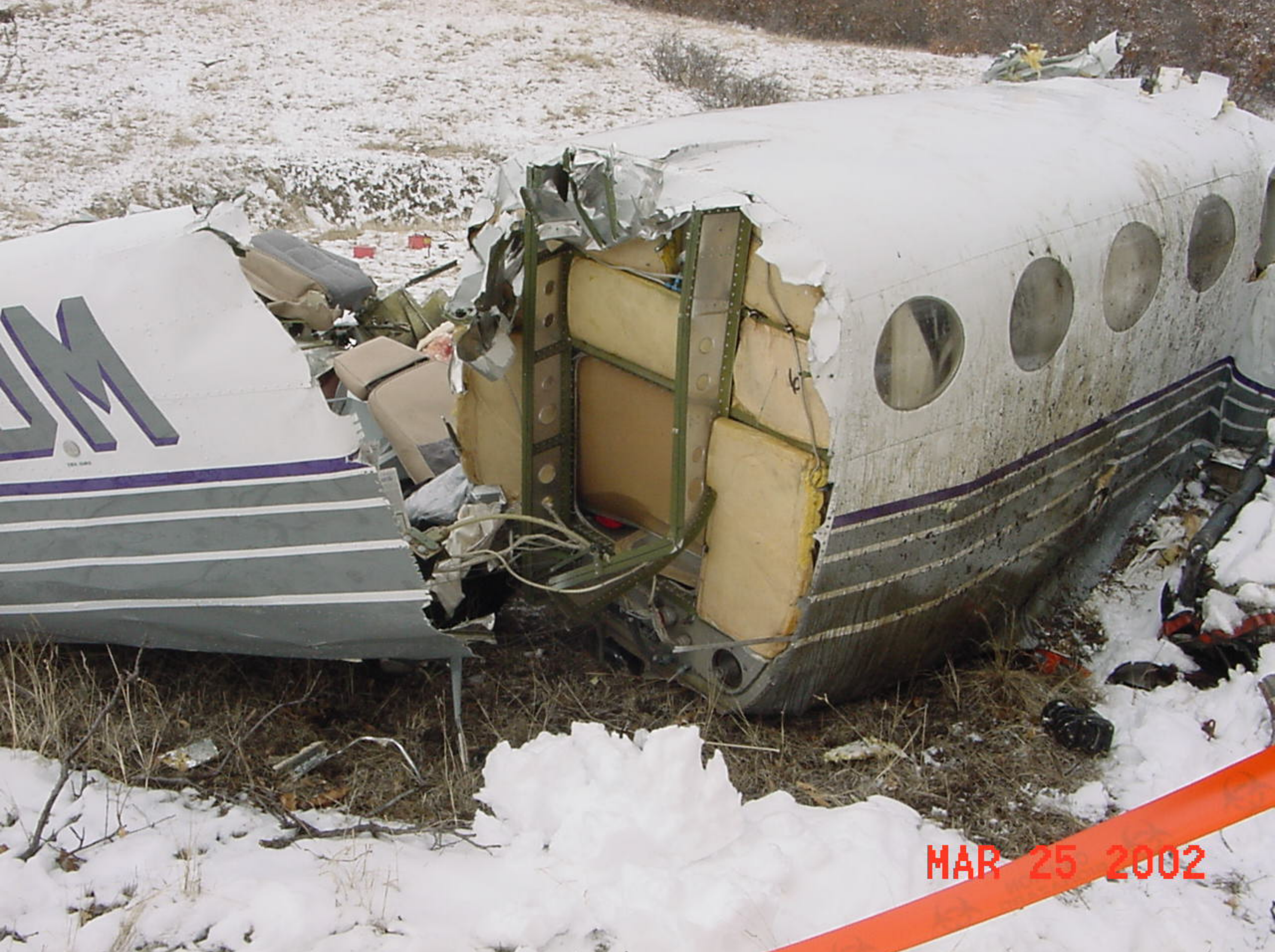
Photo #6- Separation between empennage and fuselage
