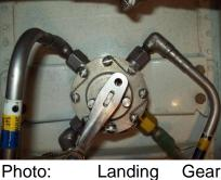
Photo: Landing Gear Selector Valve in The Full Position (Courtesy of stream)
