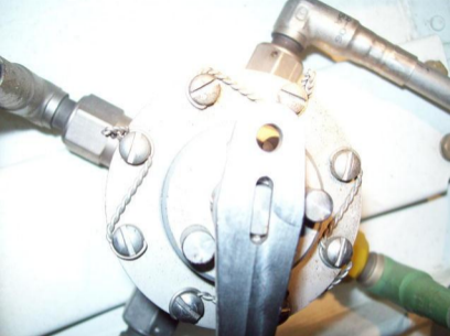
Photo: Landing Gear Selector Valve as Found (courtesy of Gulfstream)
