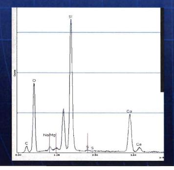
EDS Spectra from long straight fiber from E-poly coating .
