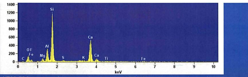
NTSB EDS spectrum of the straight fiber from N612AZ PRV contained major elemental peaks of silicon, aluminum and calcium with minor elemental peaks of iron, magnesium, carbon, and oxygen, consistent with e-glass.(direct from NTSB Materials report)
