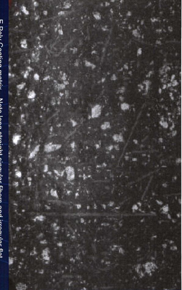
E Poly Coating matrix - Note long straight singular fibers and irregular flat pieces contained in matrix
