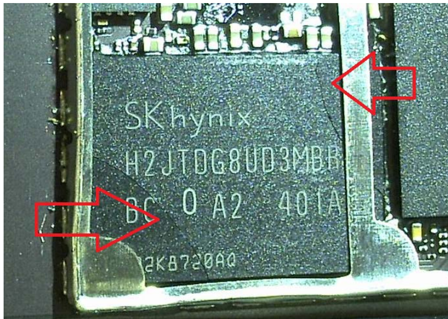
Figure 5. PED-07, non-volatile memory chip cracked.
